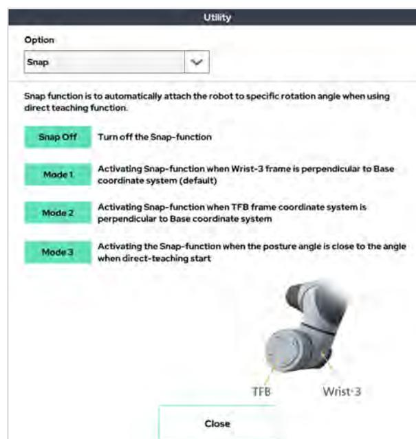
Snap mode selection window to be applied when using direct teaching mode.
