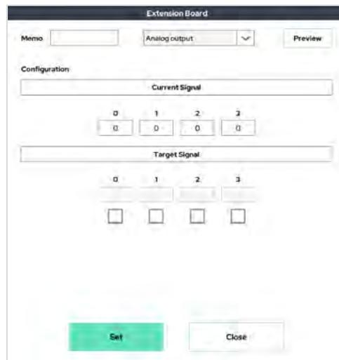
This feature controls digital/analog output when purchasing and using an extended I/O module. The method of use is the same as the existing D.output and An.output.
