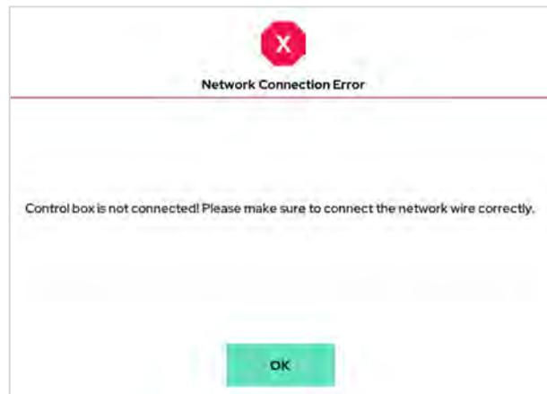
This message will occur when the Tablet PC is physically disconnected from the control box.
