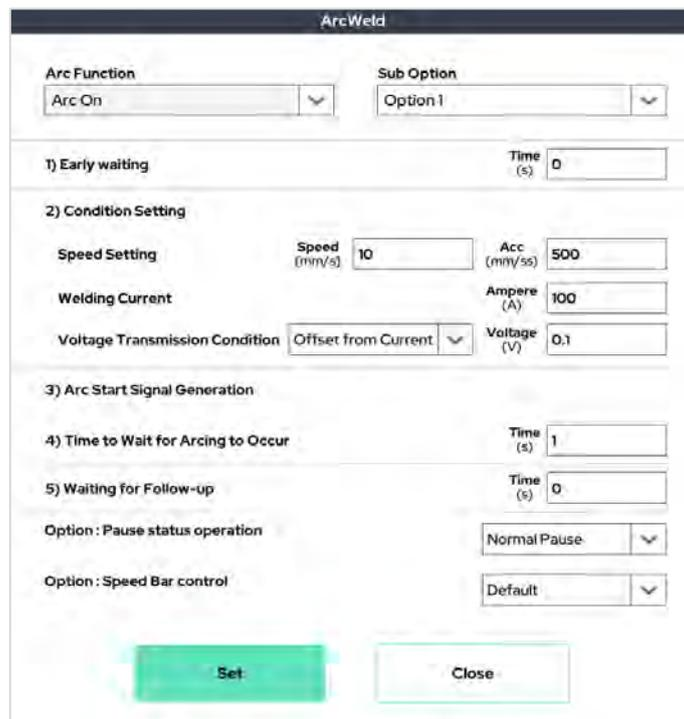
This is a special function for arc welding. A special macro function designed to quickly enable implementable functions, such as Wait / D.out.
