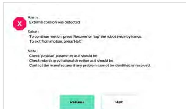
The robot will stop immediately when a collision is detected.
