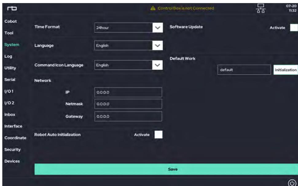
In the "Software Update" section on the right, check the Activate checkbox.
