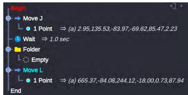
Step2) Press the Cut button. Once Cut is clicked, the line disappears from the program tree.
