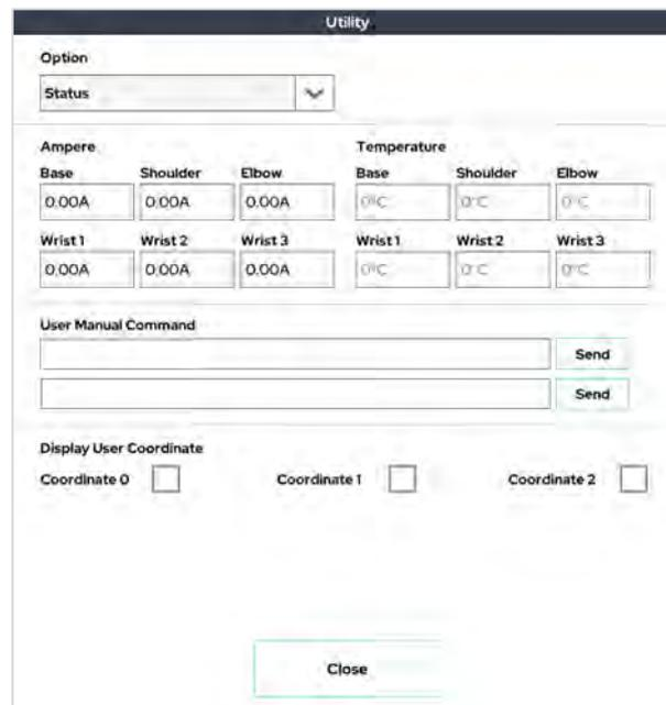
This window allows the user to see the robot arm's current and temperature. It also shows the user coordinate system settings.
