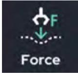
This function is used for force control. The movements below the Force Control function automatically change the trajectory to give the set force.
