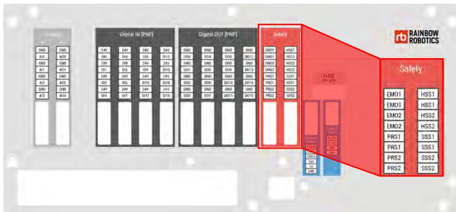
The additional ports can be equipped with 4 equipment. The robot is delivered with a default configuration, which enables operation without any additional safety equipment.
