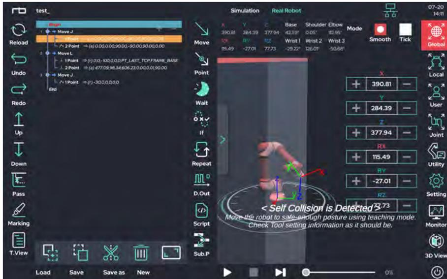
The image below shows a situation where the virtual collision box set up by the user detects / predicts a collision. The robot will stop, prompting the UI to display a warning in red.
