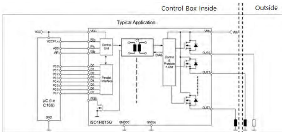
How to use RB Control Box Digital Output Device [DO00-DO15].
