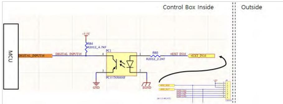
Device configuration that receives Control Box Digital input [DI16-DI17]. There is an internal 24V supply terminal. A malfunction occurs when an external 24V is supplied.
