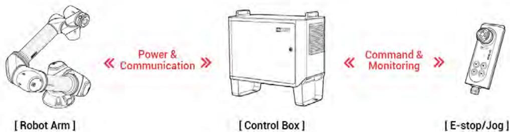
[ Stand-type control box system configuration ]
