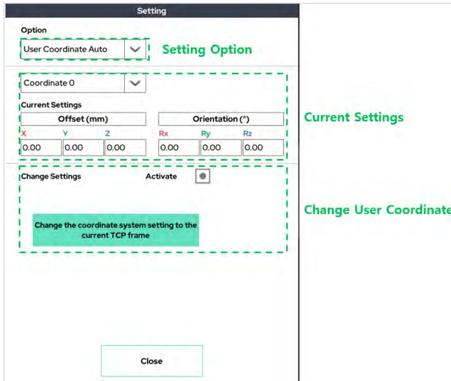
Changes the coordinate system setting to the current TCP frame.
