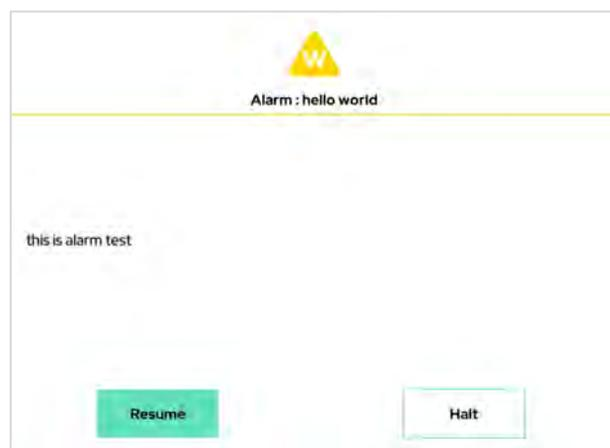
When an 'Alarm' is set in the current program, the robot will pause once the 'Alarm' command is reached. A dialog will then pop up.
