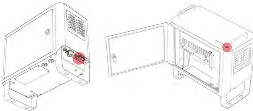
To turn off the power, press the main power switch for a few seconds.
