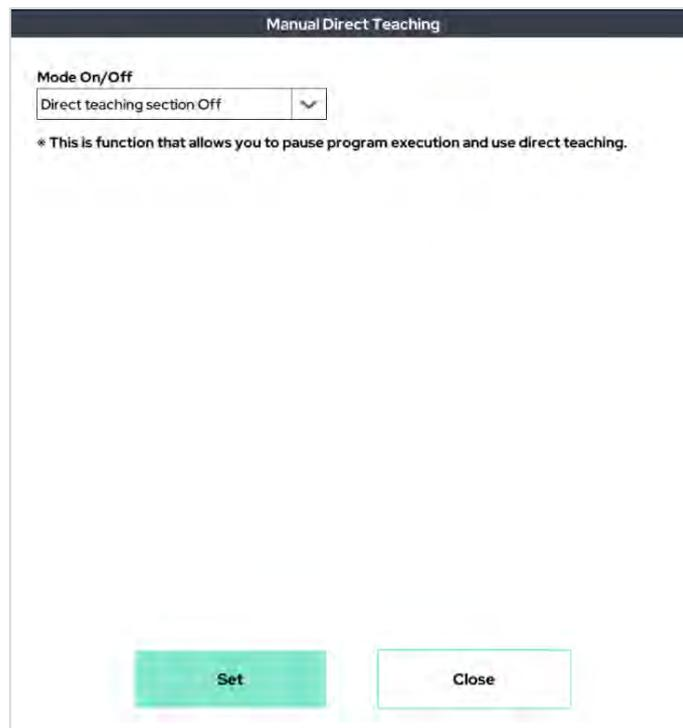
This feature enables direct teaching during program execution. For 'Mode On', the program pauses when the manual direct teaching command is executed and a pop-up window appears on the screen as shown below.
