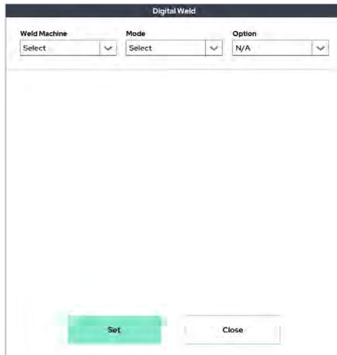
This function enables the use of the digital weld machine. After selecting the weld machine to be used, user can proceed with 'Weld Start', 'Weld Off', and 'Weld Setting'.
