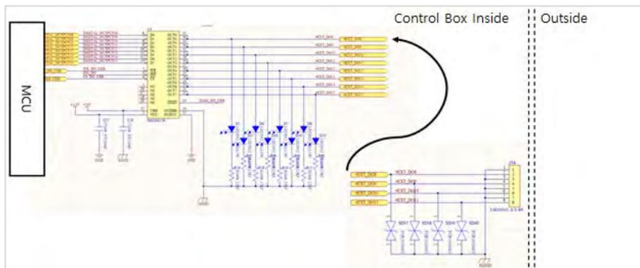
Device configuration that performs Control Box Digital output [DO00-DO15]. There is internal GND terminal, and it should be connected to GND of external sensor and equipment to be connected.
