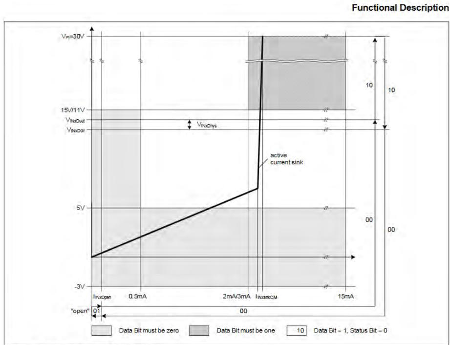
**Figure 11** Sensor Input Characteristics
