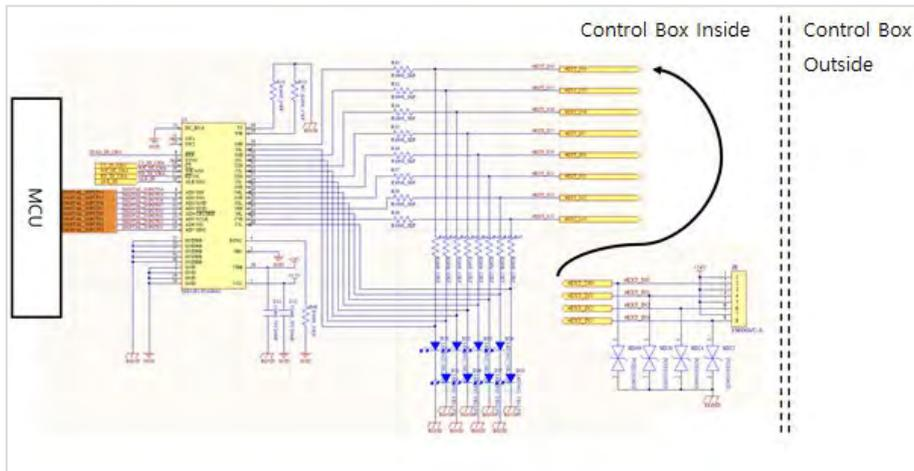
Device configuration that receives Control Box Digital input [DI00-DI15]. There is an internal 24V supply terminal. A malfunction will occur if an external 24V is supplied.
