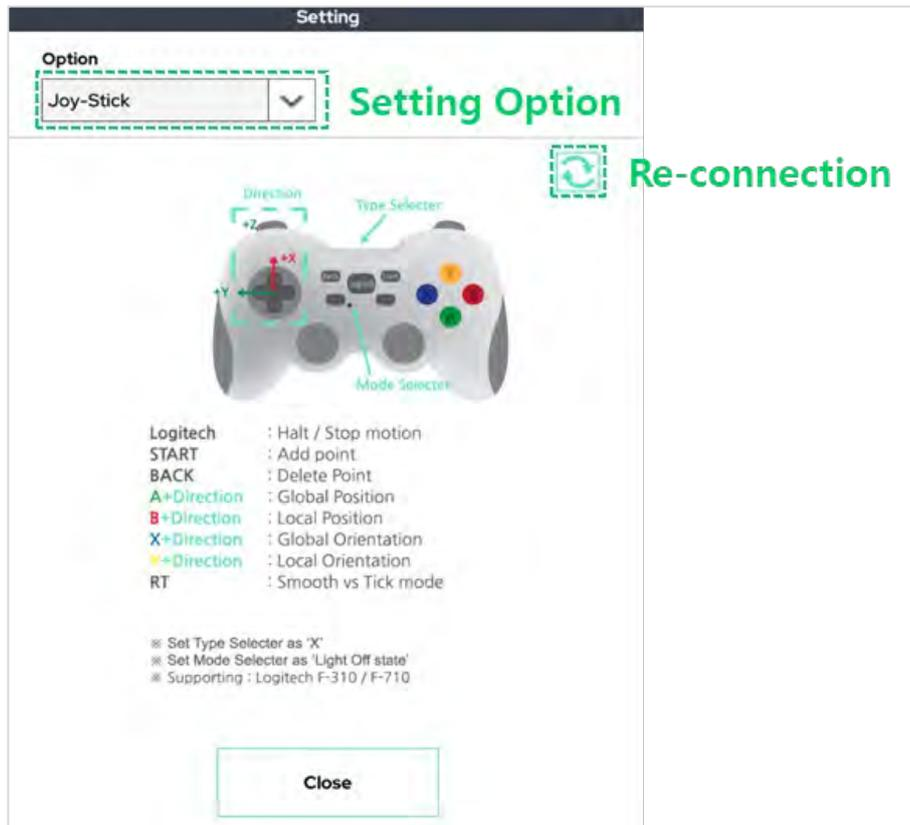
The Joystick setting allows the user to control the robot using a joystick connection.
