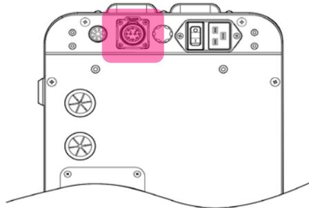
[ Connecting Part for Robot Arm cable ]
