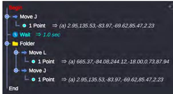
Step2) Click the Del button. The command has been removed as shown below.
