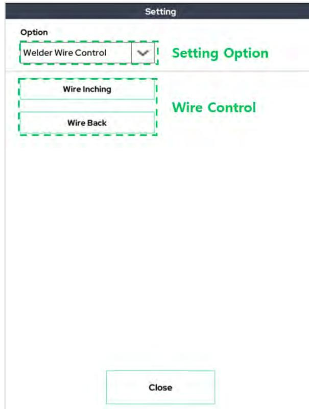
This function can control the welding machine's wire.
