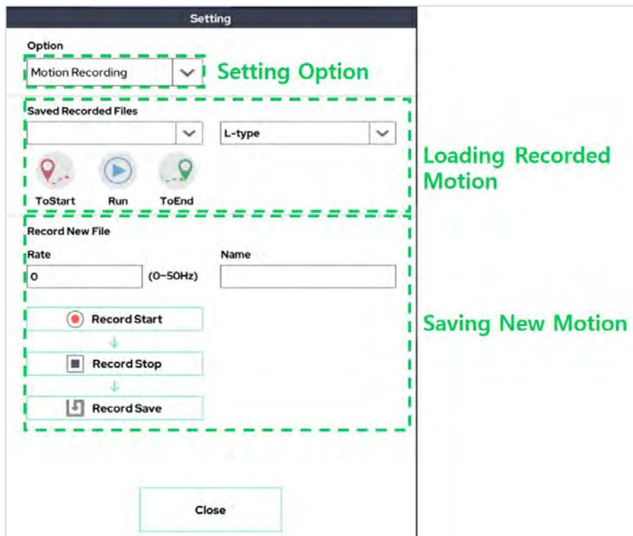
This function records the motion through the direct-teaching(gravity compensation) function. The recorded action is available in the program via the Replay function.
