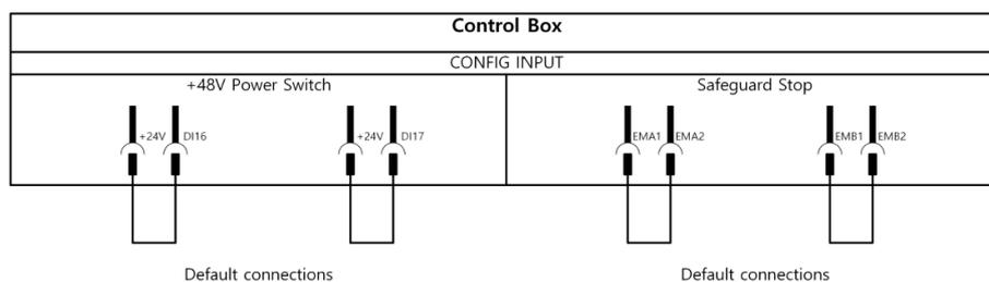
The initial factory condition is as above, and it is possible to install the operation.
