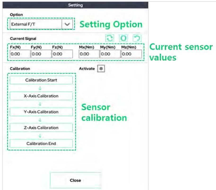
This window allows you to check and calibrate the external F/T sensor (e.g. Robotiq F/T sensor).
