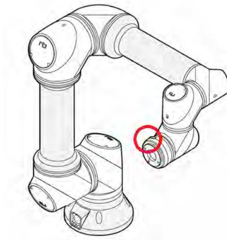
The 'gravity compensation' algorithm allows the robot to keep its pose when set by a user. For 'Direct-teaching', a user must press and hold the mechanical button located on the Tool flange. Pressing this button allows each joint to move freely. The red circle in the diagram above indicates the location of the button.
