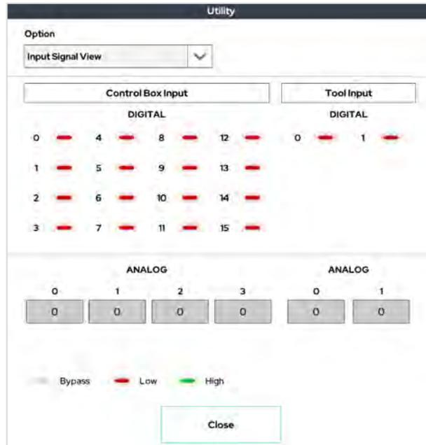
Input signal monitoring window for control box and tool flange.
