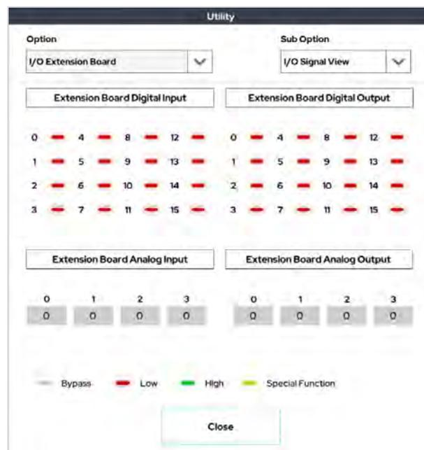
I/O expansion module's I/O signal monitoring window.
