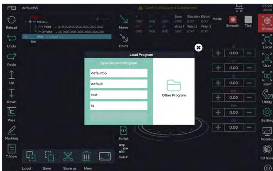
To open a file, users can click the Load option. Clicking Other Program button will open the File Explorer, which allows the user to look through saved files.
