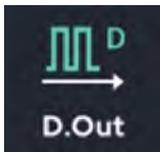
The Digital Output of the control box enables the user to select the digital output signal of whichever port (0 ~ 15) of choice. Each port has 3 possible settings: high signal, low signal, and bypass.
