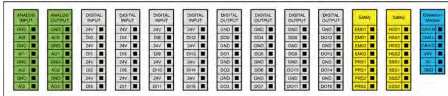
The specifications of the power and digital I / O of the control box are as follows. All digital I/O are compliant with the IEC 61131-2 standard.
