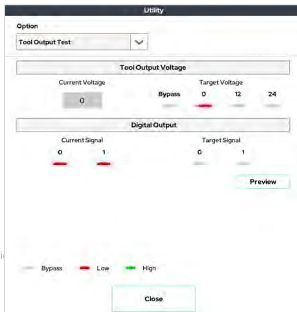
This window is used to test the output of the tool flange.
