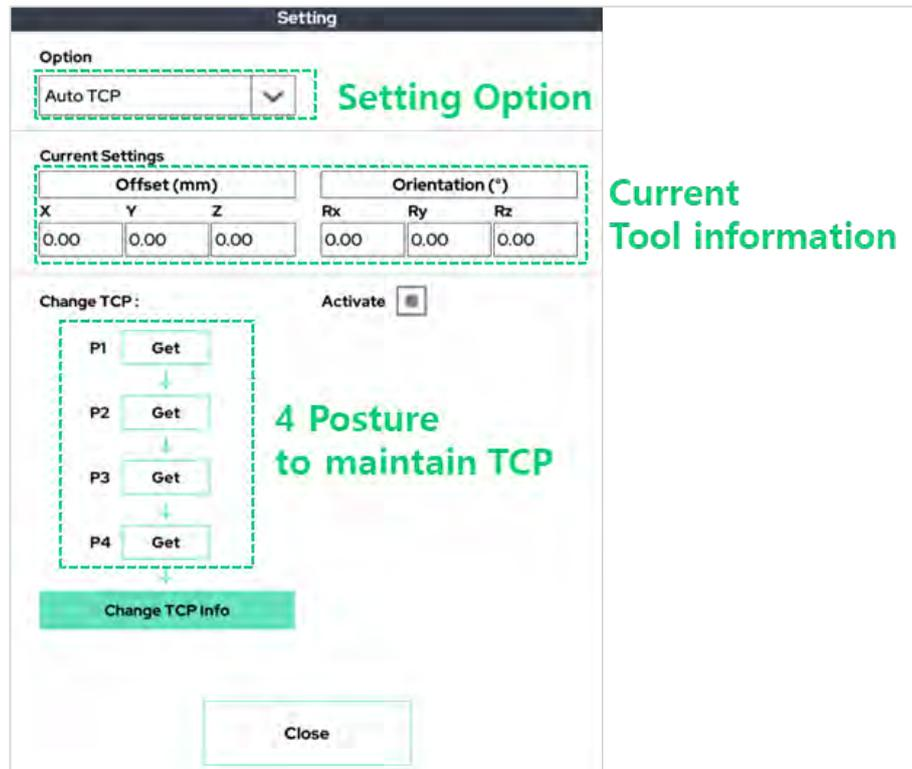
This function allows the user to find the position of the TCP automatically.
