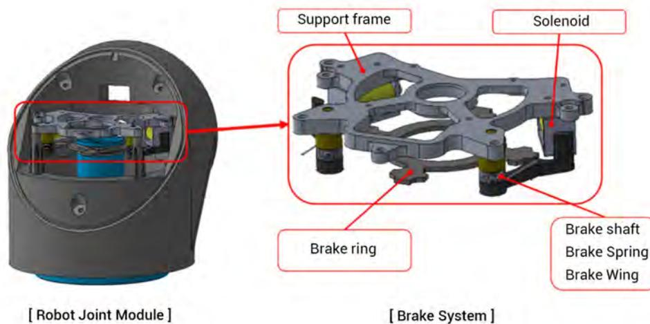
If the solenoid is on, the physical interference between the turning radius of the brake ring and the brake wing is released, and if the solenoid is off, the physical interference between the end of the brake ring and the brake wing is applied, which stops the rotation of the driveshaft.
