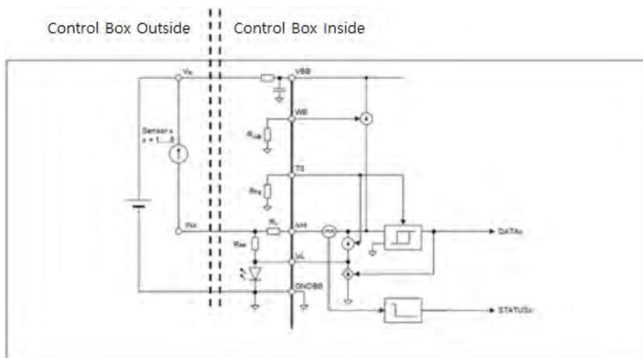
How to use RB Control Box Digital input device [DI00-DI15].
