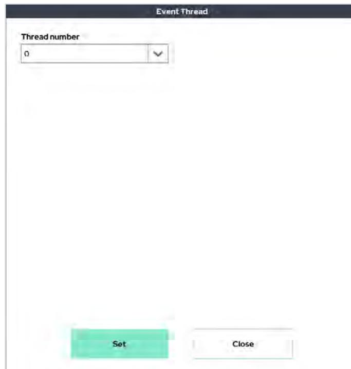
This function is used to run the event thread in the main program. The event thread is executed only when the event thread call is executed in the main program. In this case, the number of the event thread to be executed can be selected.
