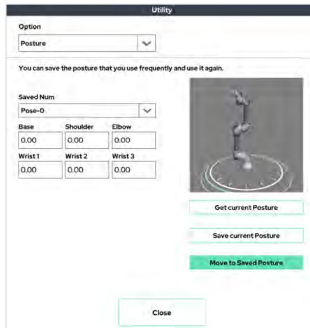
Up to 20 frequently used postures can be saved and used on the UI tablet.
