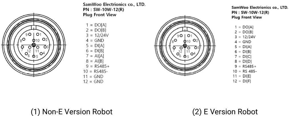
Exposed connector wiring diagram.
