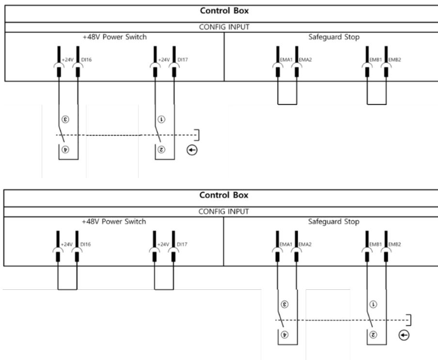
This applies to Enabling Device in accordance with ISO 10218, IEC 60204-1.
