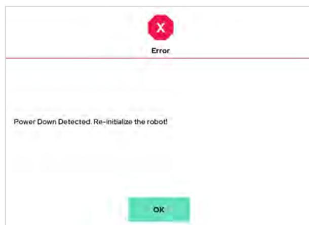
This error will appear when the robot is not receiving enough power. It may appear when the Emergency Stop button is pressed. If the button is not pressed, however, the AC or DC power line may be damaged.
