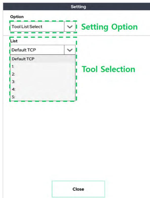
There is a Tool List Select setup feature that sets up TCP to use in a pre-saved TCP list.
