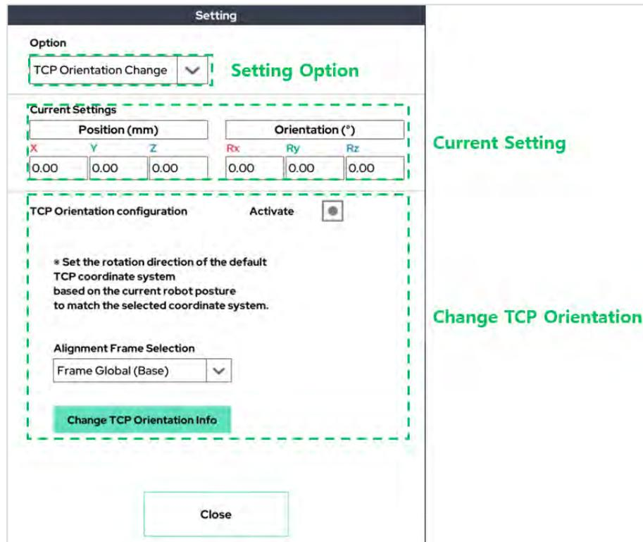
The rotation direction of the default TCP coordinate system is set based on the current robot pose to match the selected coordinate system.
