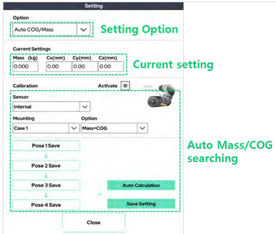
This function finds the weight and center of gravity attached to the tool using the internal / external F/T sensor.
