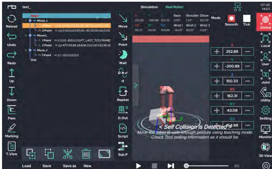
If the robot stops during operation in real mode, please move the robot arm to a safe position with direct teaching function before continuing work.
