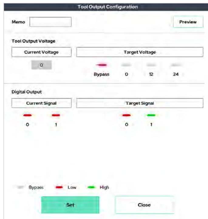
With the control box connected to the teaching pendant, and after activating the robot, set the Target Signal menu as shown above. Then press the Preview button to preview the tool flange output signal.
