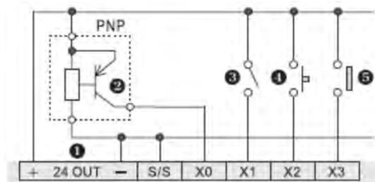
PNP sensor can be used in the same way as the above connection.
