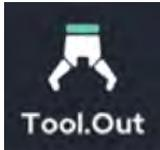
The tool flange has two digital outputs. Signals from two digital outputs can be specified. In addition, the level of voltage to be output from the tool flange (0V or 12V or 24V) can be adjusted together.
