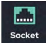
The Socket Function allows for socket communication. It provides the user the ability to open sockets to connect, send request messages, and retrieve data to/from specific server. Socket communication can be connected to at most 5 separate servers.
