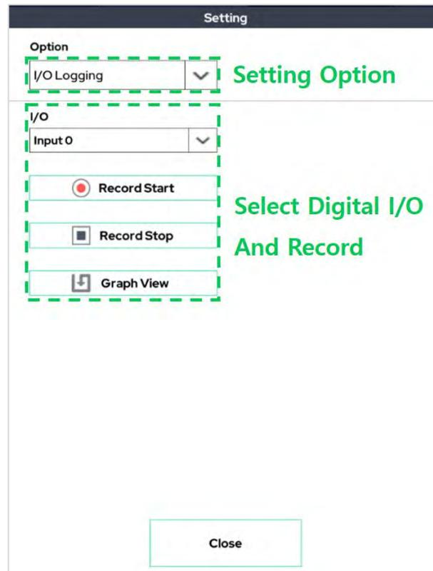
This function sets one digital input/output, records the change in the value of that input/output, and graphically shows it.
