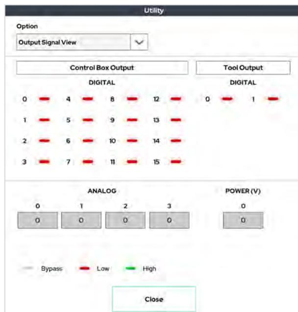
Output signal monitoring window for control box and tool flange.
