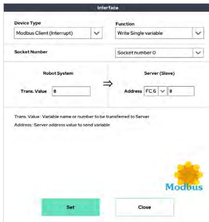
The screenshot shows a software interface titled "Interface" for configuring a Modbus Client (Interrupt) to write a single variable. The interface is organized into several sections:
