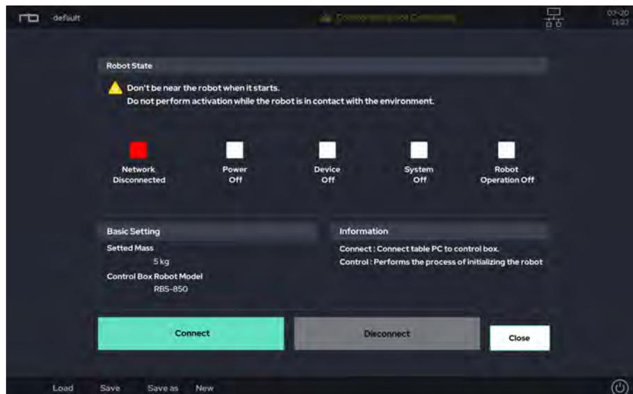
Press the "Connect" button to link the tablet PC to the robot control box.
