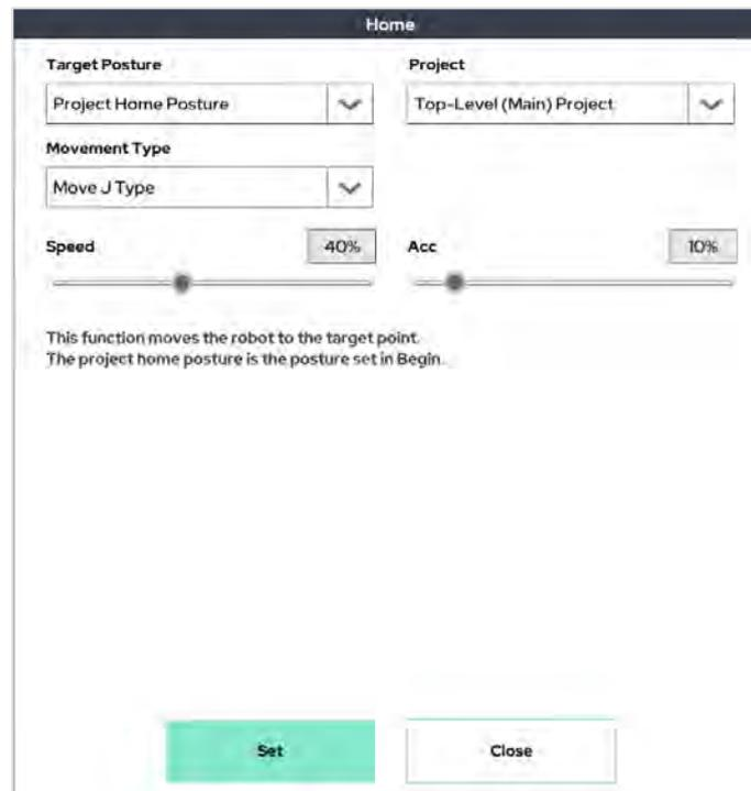
Home function is used to move the robot with Project Home Posture or Joint Zero Posture. At this time, the user can select the movement type. When going to the Project Home Posture, the user can select Project Home Posture of the main program and Project Home Posture of the subprogram.
