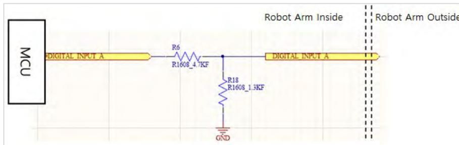
Device configuration for Tool Flange Digital input.
