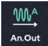
The Analog Out Function controls the analog output of the control box. Outputs the selected voltage through the target (0 ~ 3) analog ports. Each port can output a voltage range of 0 ~ 10V.
