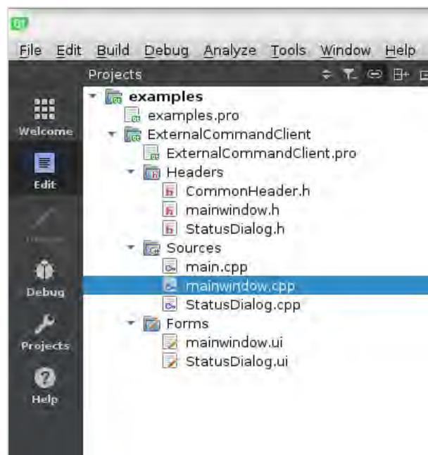
The core contents of the example are included in 'mainwindow.cpp' and 'mainwindow.h'. In 'CommonHeader.h', users can check the shape of the robot status data.
