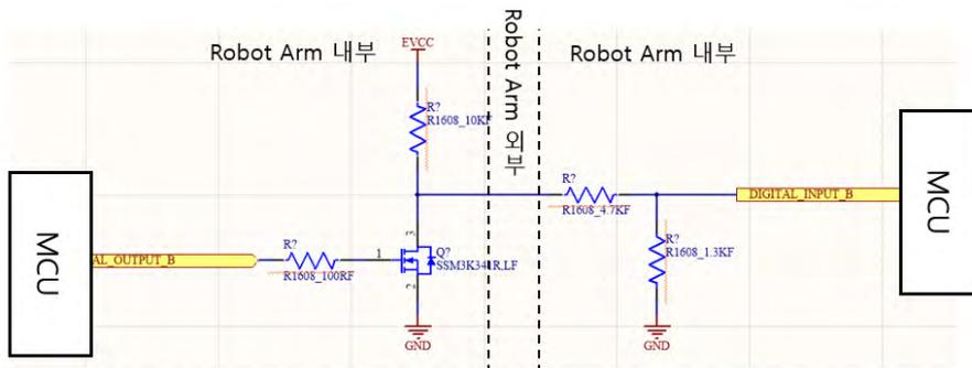
When Rainbow Robotics' digital output is connected to the digital input
